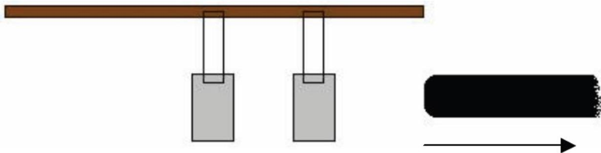
3. Use the Top and Bottom tapes to determine whether there is a net charge on each piece of foil.
