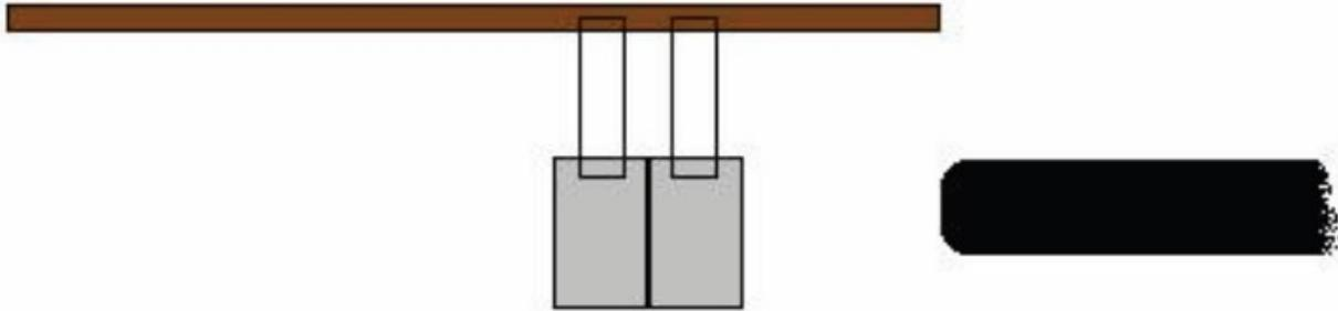
2. Bring a charged PVC pipe near, but not touching, the edge of the piece of aluminum foil. While the pipe is still near the foil, move the pieces of foil apart by touching the tape only. Then remove the pipe.
