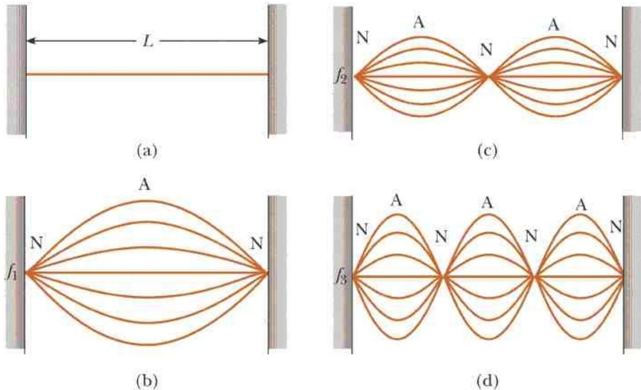
Try making standing waves like those in the image above. The figure in (b) of the image is called the fundamental and is easiest to make. What is required to establish the standing waves in (c) and (d)? How are the concepts of frequency ( $\nu$ ) and wavelength ( $\lambda$ ) being demonstrated and which changes in each of the figures? How  $\lambda$  and  $\nu$  related?
